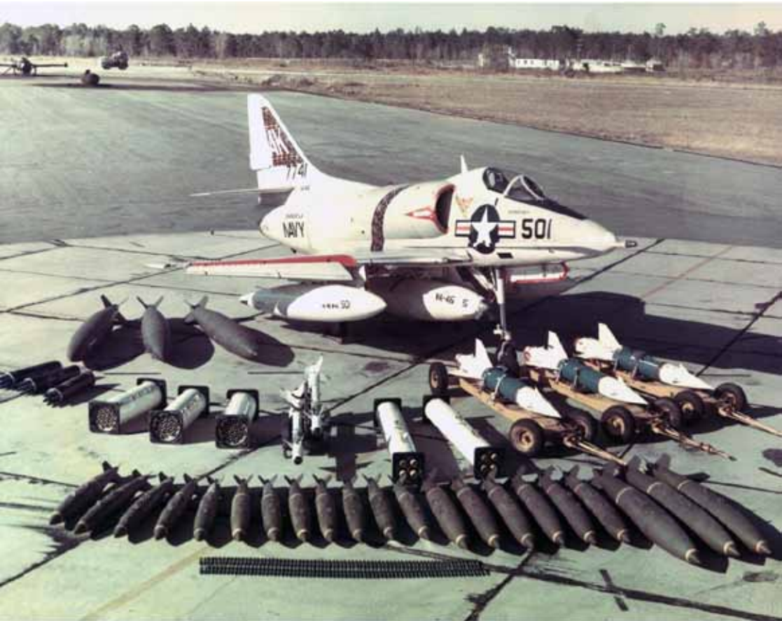
An A-4C from Squadron VA-46 (USS Shangri-La) poses with some of the ordnance which can be carried. In addition to the variety of bombs, this array includes ASM-7 Bullpup A and GAR-8 Sidewinder 1A missiles, LAU-3A/A 19-shot 2.75-in rocket packs, and LAU-10A 4 shot 5-in Zuni rocket packs. The aircraft itself is carrying two fuel tanks and a Douglas-developed D704 in-flight refueling store.
