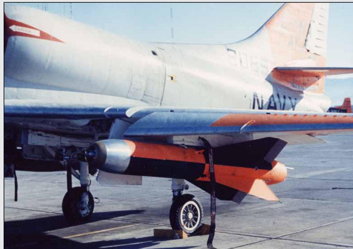
Prototype Walleye television-guided bomb loaded on A-4B 142085 for demo event 13. USN photo.
