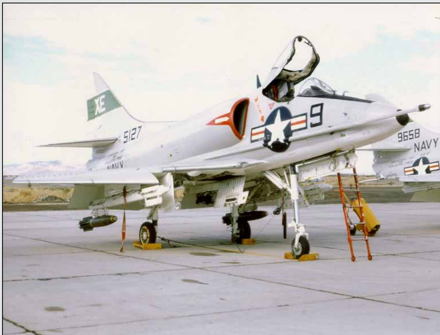
A-4C 145127 ready for demonstration event with three MK-81 bombs fitted with prototype Snakeye fins. Gary Verver photo.
