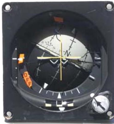
AJB-3 needle display used with the A-4 low altitude bombing system (LABS). Photo via the author.
