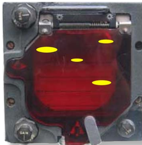
APG-53A display used with the A-4 search and terrain following radar, showing SIDS display. Photo via author.
