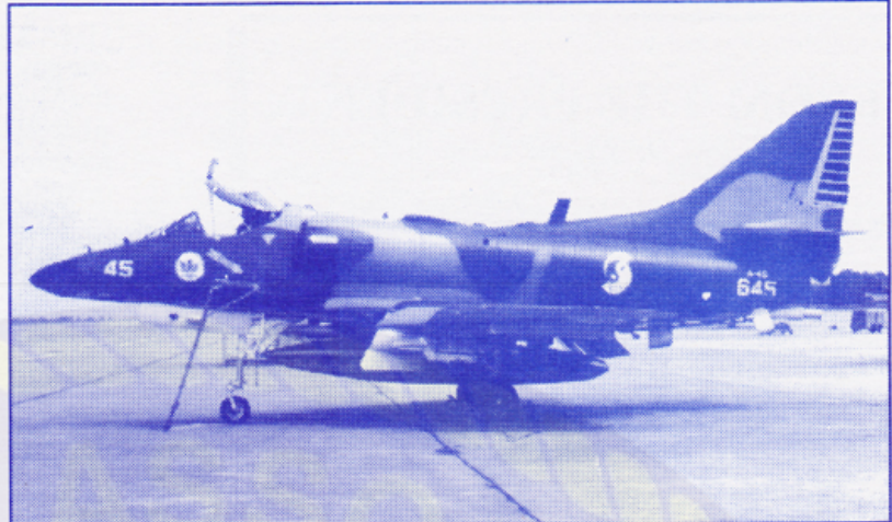
THE SINGAPORE AIR DEFENSE COMMAND received 40 A-4S aircraft (ex-A4D-2/A-4Bs) between 1974 and 1982. The aircraft were overhauled by the Lockheed Aircraft Service Company, the first eight in the U.S. and the remainder by LAS-Singapore. Overhaul included improved electronics, drag chutes, and 30mm cannons. Initial SADC pilots were trained at NAS Lemoore. In the late 1980s, Singapore undertook an ambitious program to upgrade Skyhawks to the A-4S-1 status. (Photo courtesy of Harry Gann)
