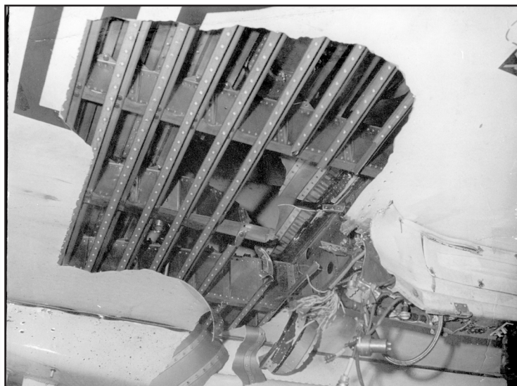
Wing damage to Pete Munro’s A-4E 151086, underside.
